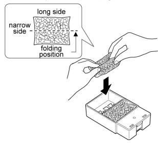
Make sure the bags not protrude from the cartridge's backside. (If the bags protrude enough to touch the motor fan, motor fan might not rotate & cause problem.)
