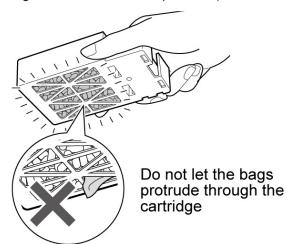
Put the cartridge back into the main body.
